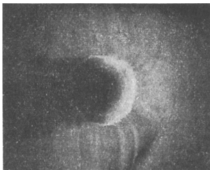
Fig. 1. Jet-like evaporation from a porous cylinder with a diameter of 40 mm.
